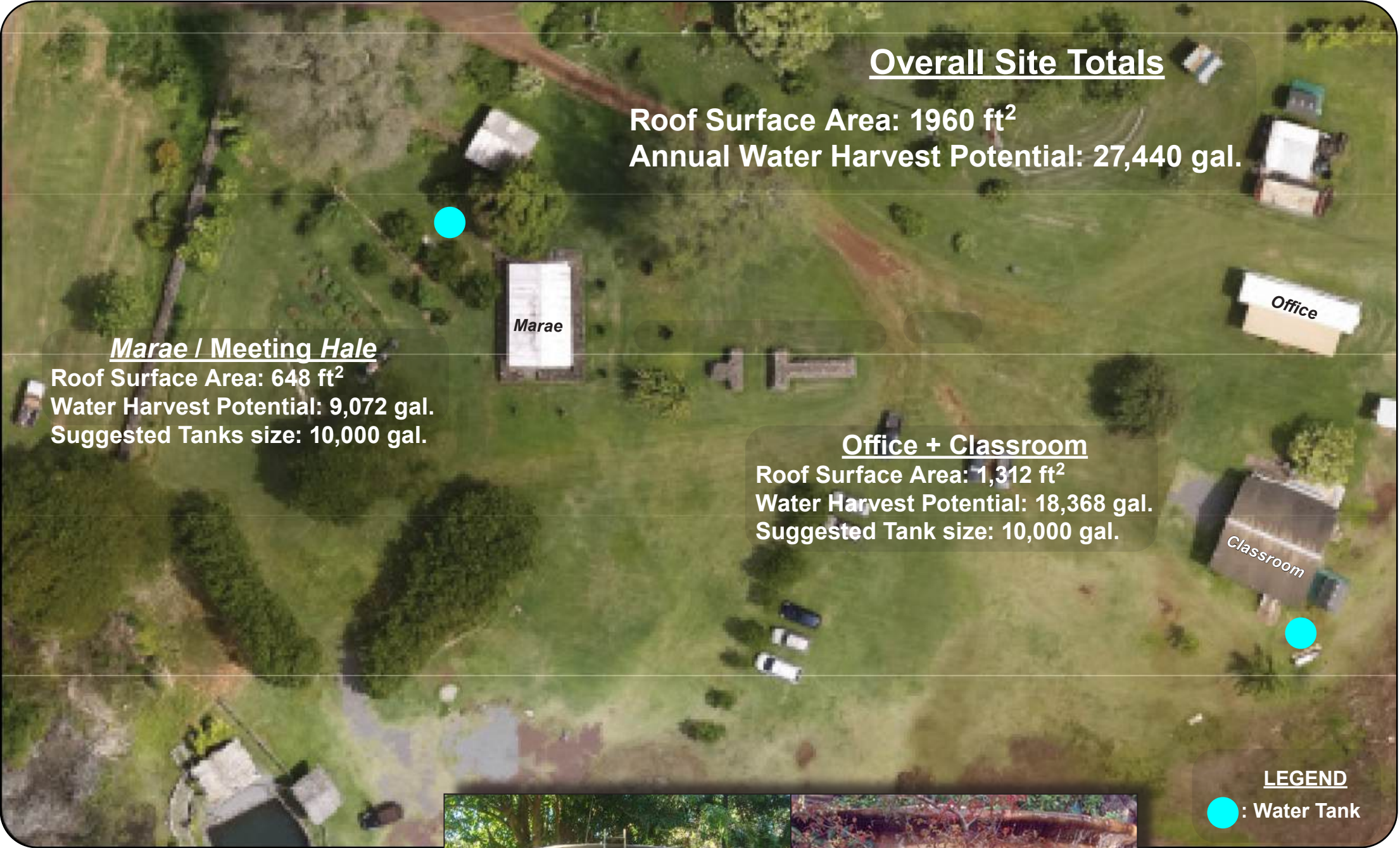
Design Detail A: Rainwater Catchment Schematic
